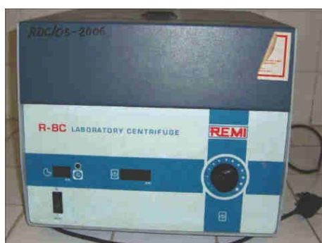
Figure 1: Centrifuge machine used for preparation of Platelet-rich fibrin from blood samples in the vacutainer tubes.
